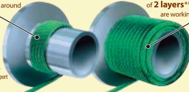
\*\* Pulling capacity is determined by the load a winch can pull with only the bottom layer of rope on the drum. For practical purposes, full capacity is retained with up to 2 layers.
